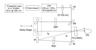
Fig. 1. Experimental setup.
