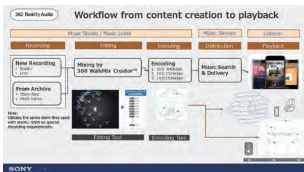
Fig. 4 The workflow of 360 Reality Audio
