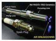
**Fig. 1.** Photograph of a laser igniter and current spark plug. This figure was already published and therefore its reference should be shown cleary [1]. The format of the reference is explained in the 5<sup>th</sup> section in this style-guide.
