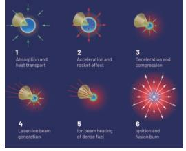
Direct-Drive, Proton Fast Ignition using a cone-guided capsule
