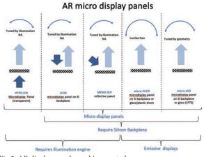
Fig.2: AR display panels used in smart glasses
