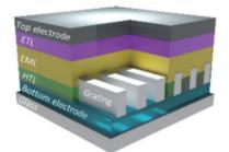
Fig. 1: Schematic representation of a) OLED and b) OSLD.
