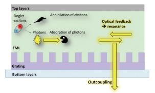
Fig. 2: Illustration depicting the exciton and photon losses as well as optical feedback and outcoupling in an OSLD.
