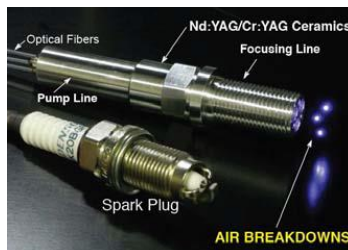
Fig. 1. Photograph of a laser igniter and current spark plug. This figure was already published and therefore its reference should be shown clearly [1]. The format of the reference is explained in the 4 th section in this style-guide.
