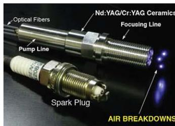
**Fig. 1.** Photograph of a laser igniter and current spark plug. This figure was already published and therefore its reference should be shown clearly [1]. The format of the reference is explained in the 5<sup>th</sup> section in this style-guide.
